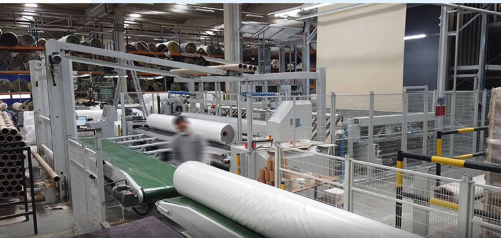
The line includes, amongst others, 4 accumulators as the crucial buffers between a continuous and a non-continuous process, an in-line inspection and re-work section, a fully automatic roll-up unit and an automatic wrapping dispenser as well as an automatic paper core dispenser for various film and tube sizes. All machinery is connected via guiding sections, including intelligent material-steering technology for straightly wound finished rolls of various qualities.
