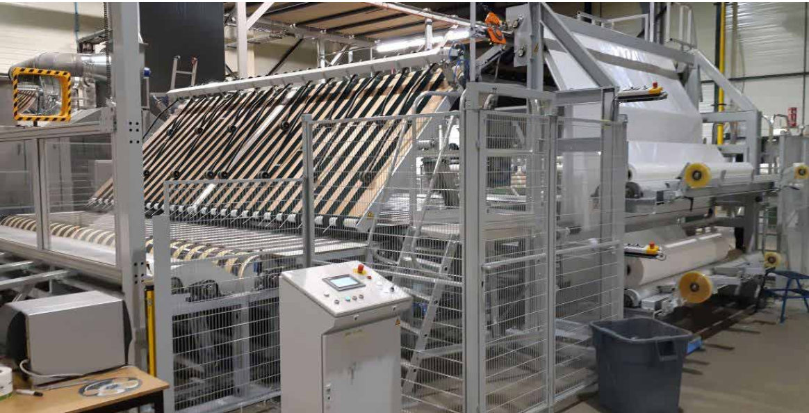
M 5220 Off line wrapping machine artificial grass ETF Automatic wrapping machine for offline wrapping of mummified rolls of artificial grass with large diameters.
